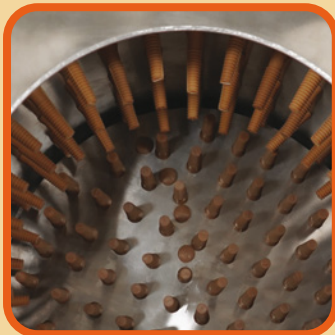
Drum has 196 plucker fingers for max efficiency
